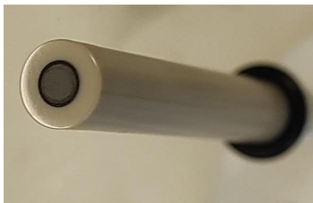
Figure 32. Photograph of inhomogeneous catalyst thin film obtained on a GC electrode after drying the catalyst ink in air. Catalyst: AI004Cat.
