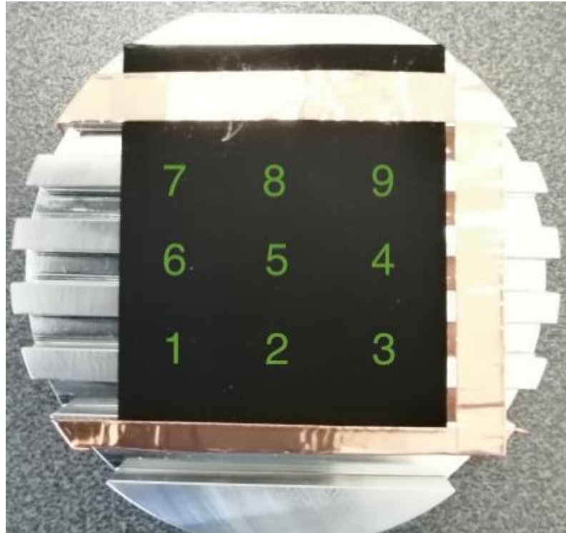
Figure 20. Arrangement of EDS scanned windows on the surface of ready GDE.
