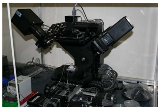
Figure 2: Woollam M2000-DI Spectroscopic ellipsometry
