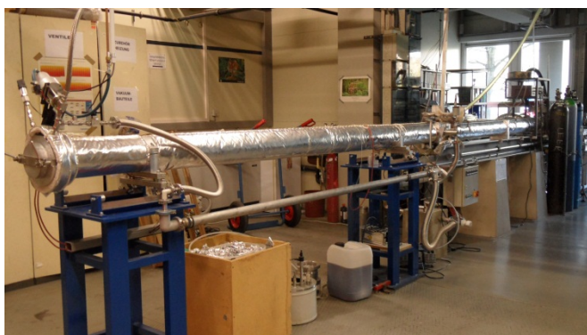
Figure 1 The shock tube apparatus (ST)
